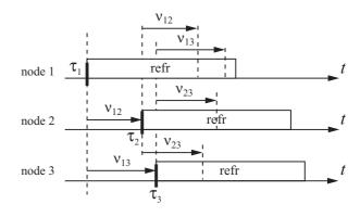
Fig. 3. Synchronization interactions for three nodes connected all-to-all.
