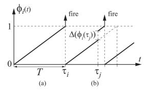
Fig. 1. (a) Uncoupled PCO phase function and (b) Phase increment upon reception of a pulse.
